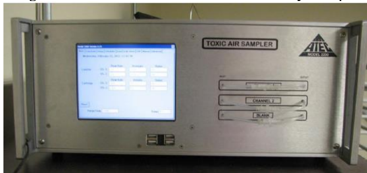
Figure: ATEC model 2200 2-channel carbonyl sampler
