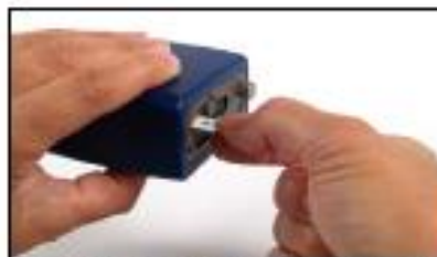
Figure 9: Inserting and removing filter strip while depressing filter release button on bottom of microAeth.
