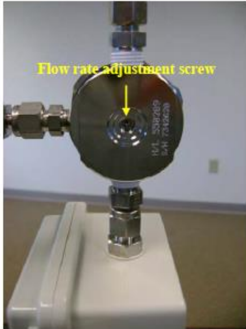
Figure 4. Flow rate adjustment screw
